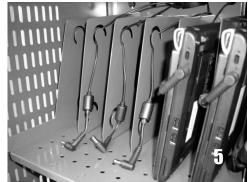
Thread computer plug cable through the holePull the computer plug cable through the front slot and Thread the cable through the loops so that the plug is in the correct position to attach to the computer, as shown. Below is a detail of the divider panel showing the loops.
