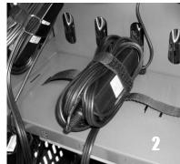
Wrap the Cord Set with both cables around the adapter as shown, leaving 16" for computer plug, 8" for power plug. Lay the wrap on the Velcro strap as shown.
