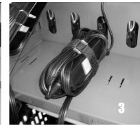
Buckle the Velcro strap around the wrapped cord set, cinching it down against the shelf. Velcro Buckle locks into place as shown.
