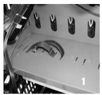
Thread the Velcro strap through the two slots directly behind the front computer slot, tacky side out, as shown.
